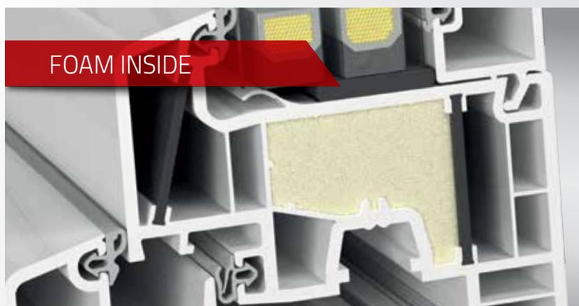
Further improvement of the thermal performance of the window by optional filling of the chosen internal profile chambers with polyurethane foam, after welding of the window construction.
